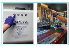
Activate the system by pressing Button 1 (or Button 2 for multiple lines). Note - If desired, you can serve the beer remaining in the line.
