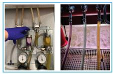
When running a clean, purge the FOB (mid cycle) by pressing it down to remove any air bubbles and get a superior FOB clean!
